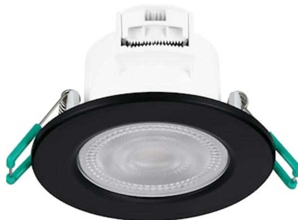
Integrated LED recessed spotlight, vertical tilt 30°, RAL9016 colour, 450lm, 6.0W, phase dimmable, 2700K/3000K/4000K, 38° degree beam angle, ABS plastic white body, low profile 47mm recessed depth, IP44 from the front, IK03, loop-in/loop-out terminals for fast wiring, 87mm bezel diameter, 68-74mm cutout, clear lens.
