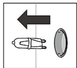
5. Screw the new illuminant in. Check its proper position in the socket.
