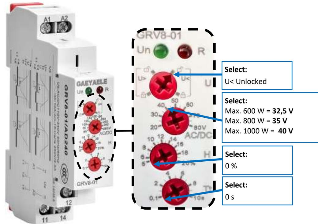
The **GRV8-01** is the main control unit of the automatic storm control system. It constantly measures the DC operating voltage of the turbine and immediately activates the GRT8-B1 time delay relay once the critical max. voltage of 40 V DC is reached. The control unit must be set-up as described below:
