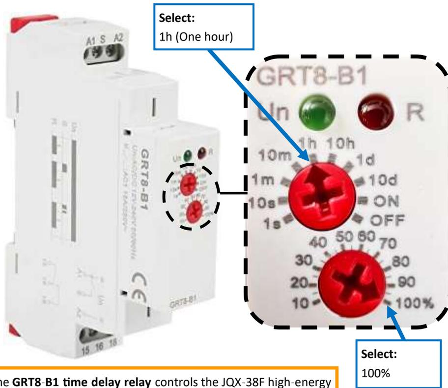
The **GRT8-B1 time delay relay** controls the JQX-38F high-energy relay which stops the turbine. It must also ensure that, once the automatic storm control has been activated, the high energy relay does not restart the turbine before the cool-down time of 60 minutes has elapsed.
