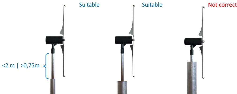
Contact a professional if you are unsure which tower to choose. Often lighting poles are used as a cost effective solution with great success. Consider the [turbines resonance frequencies of ca. 10 - 50 Hz](#) depending on load and rpm. Immediately stop the wind turbine and modify your tower (e.g. with tension ropes) should you find that your tower is resonating! Any damage caused by excessive vibration and fatigue are not covered by the products warranty.
