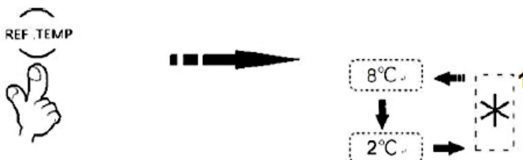
3. After a few seconds without using any operating buttons, the FAST-COOLING MODE will be activated.
