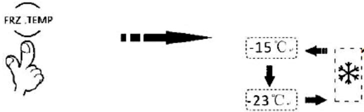
3. After a few seconds without using any operating buttons, the FAST-FREEZING MODE will be activated.
