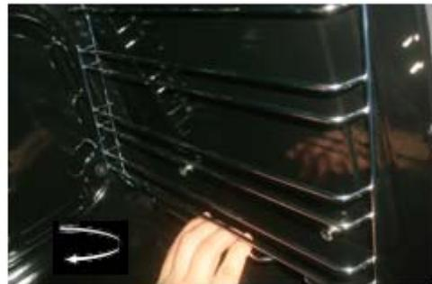
2. Hold the guide vertically to remove it from the oven.
