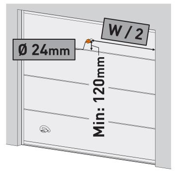
**1.2)** Position the parts of the external unblock. Unfold the cable attached to the end of the cylinder. Guide the cable through the 24 mm diameter hole, from the outside of the door. Insert the lock and align it with the edge of the door.
