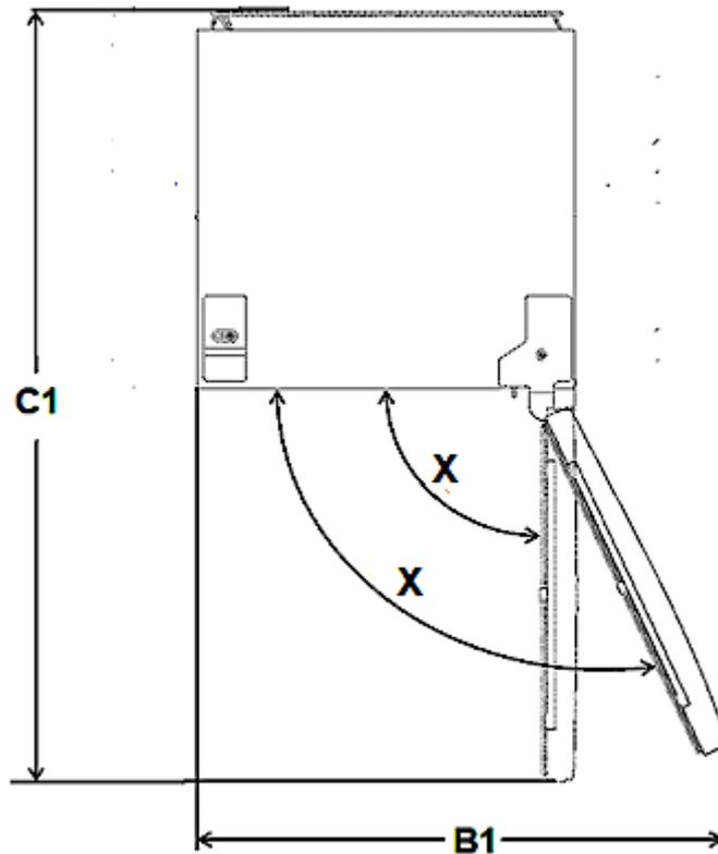
**B1 = WIDTH / C1 = DEPTH / X = DOOR OPENING ANGLE**
