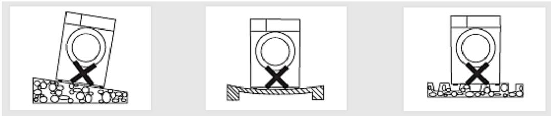
10. If you install the appliance on a wooden floor, you must also place it on a plywood panel (60.00\*60.00 cm) **at least** 3.00 cm thick to distribute the weight of the appliance. Fix and secure the plywood panel properly to the wooden floor.
