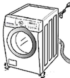
a. How to **raise** the appliance: turn the adjustable feet **to the left** (s. fig. on the right).
