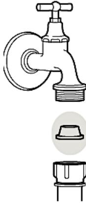
5. Reinstall the water inlet filter in the hose end. Ensure that the seal (rubber washer) is properly inserted in the valve connection.
