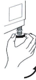
**NOTICE!** After you have levelled the appliance properly, always tighten the lock nuts again.
