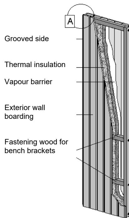
**Before installing the individual panels, ensure that the grooved side (viewed from outside) is always located on the left.**
