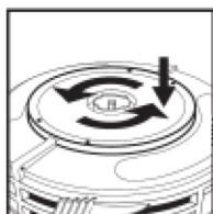
fig. 7 - fit new side plate
