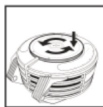
fig. 12 - fit side plate
