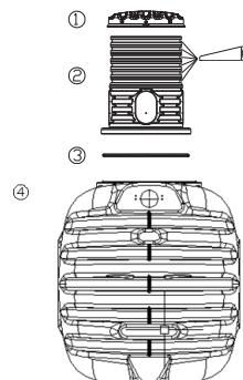
The shaft extension can be shortened at the grooves. This allows the soil coverage above the tank shoulder to be 400-780 mm.
