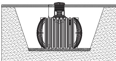
The tank must not be installed under areas of traffic.
