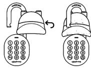
Pull and fold the silicone case down to ensure it covers the whole padlock.
