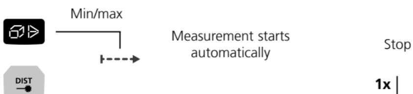
The LC display shows the max value, the min value and the current value.
