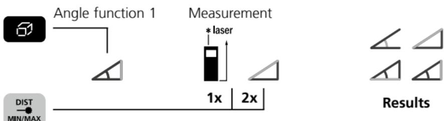
The measurement results are determined automatically by the 360° inclination sensor.
