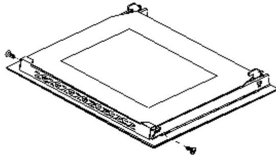
3. After cleaning, insert and block the glass panel.
