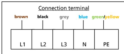
Make sure that all wires are firmly connected to the connection terminal.
