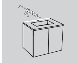
Make sure you put in a water seal between the furniture unit and the wall
