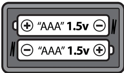
Insert correct battery type as shown in diagram inside battery compartment.
