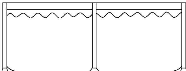
1. Make sure the drain fitting is plugged securely and the cap is in place. Start filling the pool with water. After about 1-inch of water is on the bottom, stop filling and smooth wrinkles out of the bottom of the pool. Pull the outer wall out from under the top ring, all around the bottom of the pool, so that it fills evenly.
