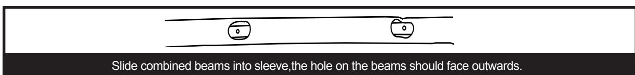
Slide combined beams into sleeve, the hole on the beams should face outwards.
