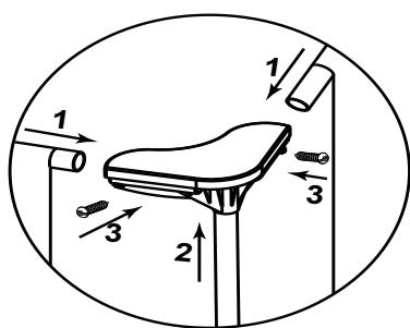
1. Use the connection end of the L-JOINT to connect the adjacent horizontal tubes.
