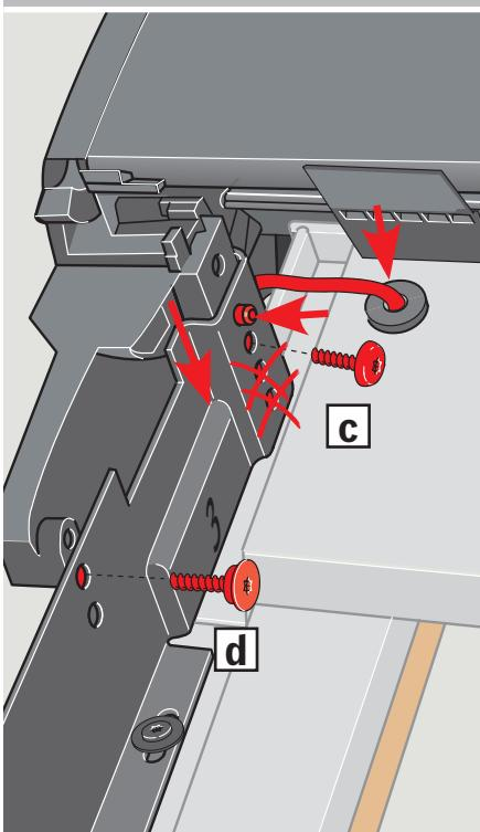
**ENGLISH:** Lower the roller shutter top casing as much as possible. Do **not** press the top casing against the roofing material **[a], [b]**. Pull cable through hole on window top cover. Fit securing screws after installing the roller shutter top casing **[c], [d]**.
