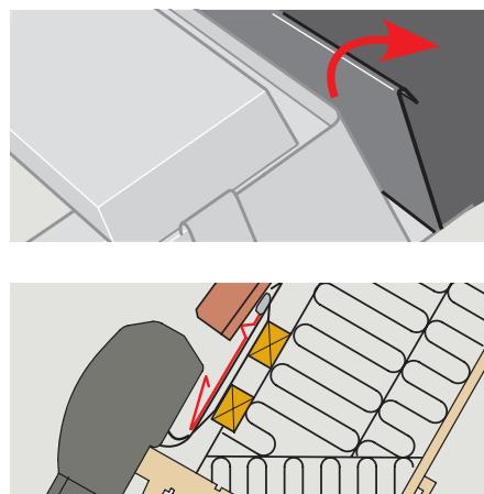
**ENGLISH:** If the roller shutter is to be installed with flashing EDJ or EDN: Bend down rainwater deflector to make room for roller shutter.
