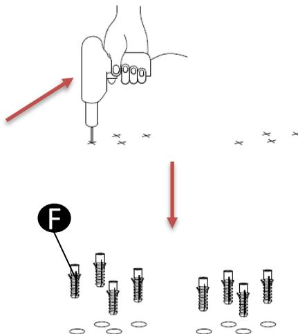
If the floor is a wooden floor,you don't need to knock in the plastic expansion pipe(REF F), use self tapping screw (REF E) to knock in the floor directly.
