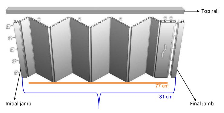
After installed, the width is 81cm (from Initial jamb to Final jamb) when folding door is closed. Top rail we provided is 81cm too.
