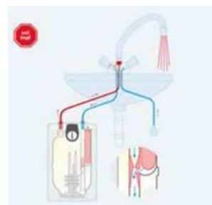
Only if water continues to drip from the tap with the boiler off and the valve closed would there be a defect in the tap.
