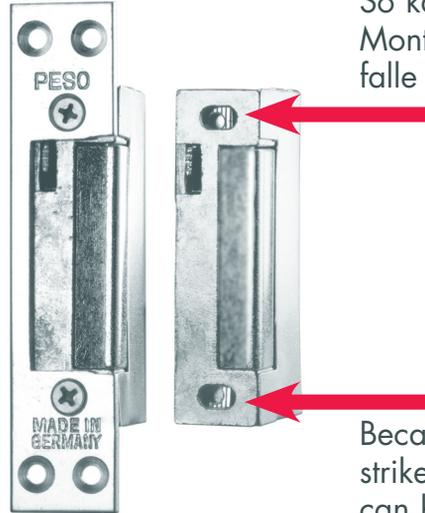
Because of the long holes in the strike casing the striking plate can be horizontally adjusted up to 4 mm. This way the strike can easily be justified towards the strike latch when installed.
